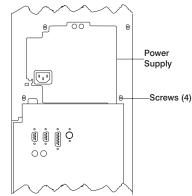
10. Remove the retaining screws that secure the power supply to the top of the system unit.
