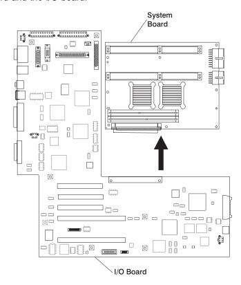
13. Carefully remove the system board from the system unit.
