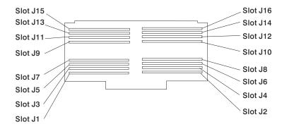
7. Remove the memory module by pushing the tabs out on the memory connectors.
