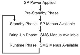
Pre-Standby Phase: This phase is entered when the server is connected to a power source. The server may or may not be fully powered on. This phase is exited when the Power-On Self Tests (POSTS) and configurations tasks are completed.
