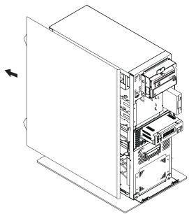
5. To remove the top cover, remove the screw at the front and the two screws at the rear and lift the cover off. (The side covers must have been removed previously).
