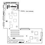
4. Use one finger to slightly slide the battery toward the front of the server. (The spring mechanism behind the battery pushes it out toward you as you slide it forward.) Use your thumb and index finger to hold the battery as it pushes out of the socket.
