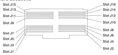
**Note:** Memory modules must be installed in pairs and in the correct slot configuration. (Slots J1 and J2, J3 and J4, J5 and J6, etc.)
