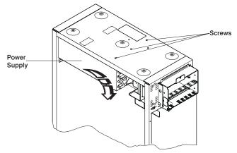
Attention: When removing the power supply ensure that the power supply does not drop down and damage the I/O board components or connectors.
