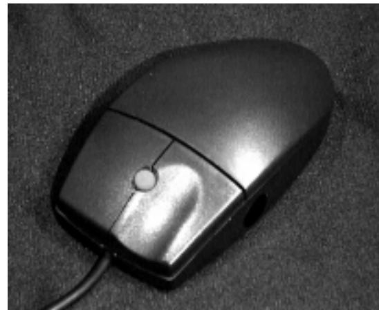
Figure 1 The JoystickMouse (JSMouse) is a mouse with an miniature joystick mounted between the two buttons. The users may use index or middle finger to manipulate the joystick.
