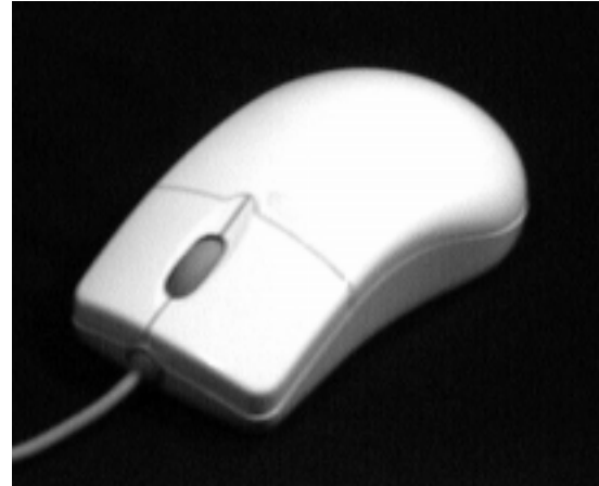
Figure 2 The WheelMouse used in the study was a Microsoft IntelliMouse™. It works in three modes: Wheel rolling, press (the wheel) and move (mouse) to do rate control, and click and move.
