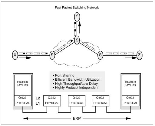
Figure 19. Fast Packet Switching Using Frame Relay
