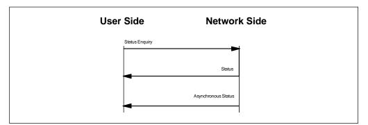
Figure 27. Asynchronous LMI Support
