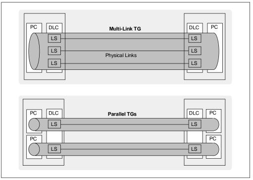
Figure 14. Multilink and Parallel TGs
