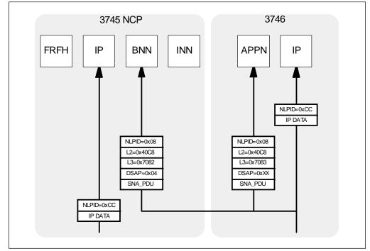
Figure 62. 3745 and 3746 IP over Frame Relay
