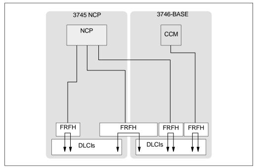
Figure 226. 3746 Frame Switching
