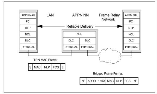
Figure 59. HPR over Frame Relay Example
