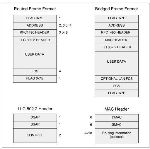
Figure 44. Routed and Bridged Frame Formats
