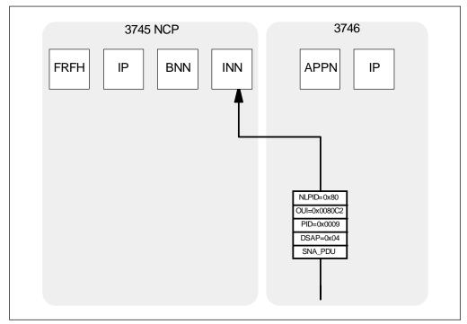
Figure 64. 3745 INN Traffic - Bridged Frame Format
