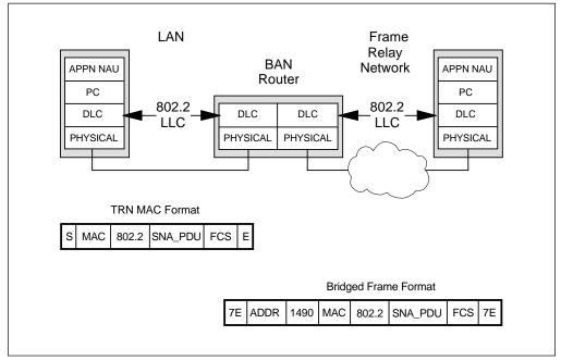
Figure 58. Frame Relay BAN Router
