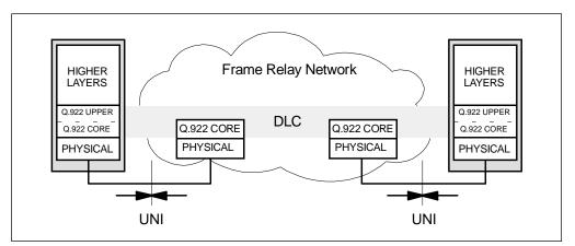
Figure 22. Frame Relay Reference Model
