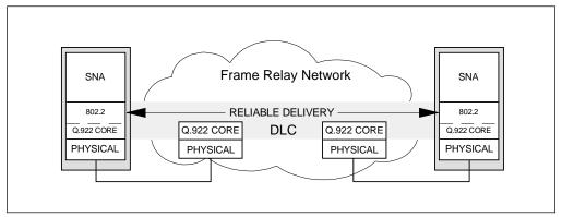
Figure 47. IBM SNA over Frame Relay
