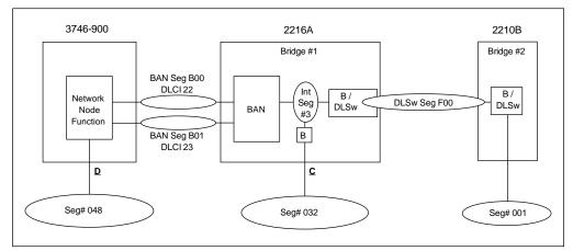
Figure 171. Frame Relay BAN Logical View
