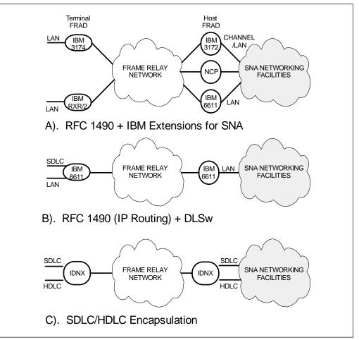
Figure 37. IBM Frame Relay Access Devices
