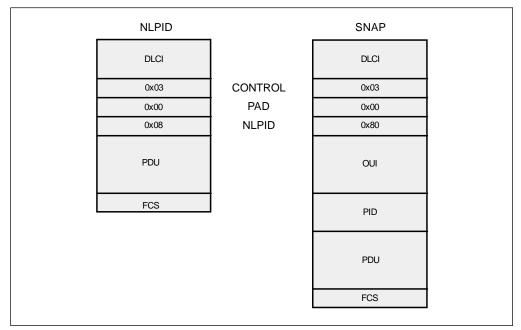
Figure 33. RFC1490 Encapsulation
