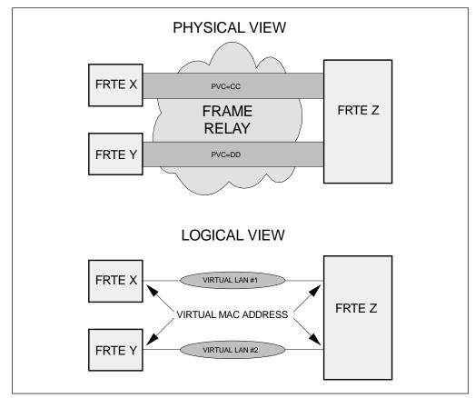
Figure 34. Bridged Frames Using a Virtual LAN
