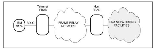
Figure 36. SDLC Frame Relay Access Device
