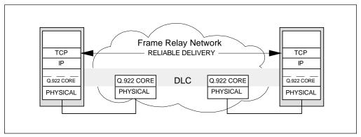
Figure 55. IP over Frame Relay
