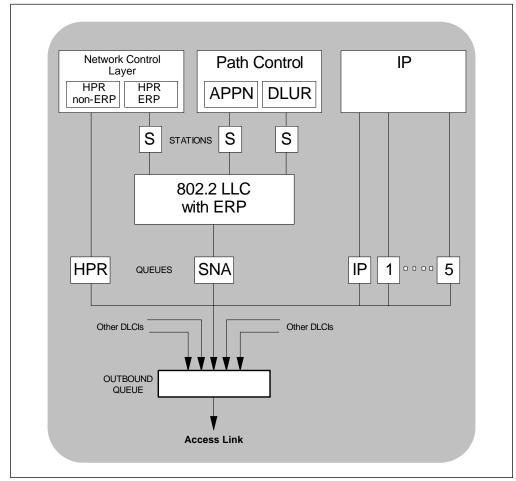
Figure 68. 3746 Frame Relay BRS
