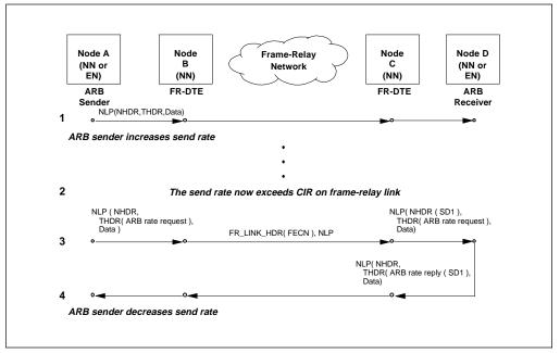
Figure 60. Intermediate Subnet Causing ARB Send Rate Reduction
