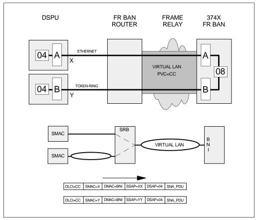
Figure 51. IBM 374X BAN-1 DSPU Support
