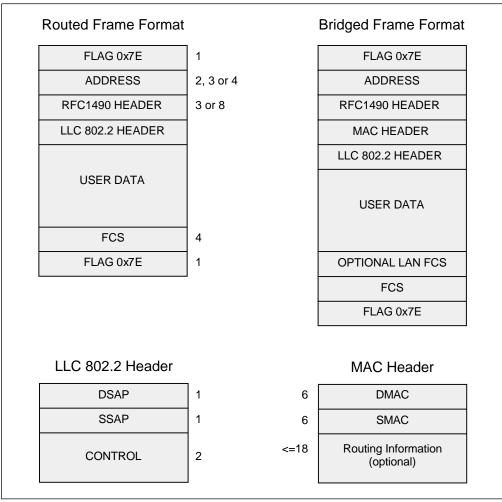
Figure 236. IEEE 802.2 LLC Protocol Data Unit Encapsulation
