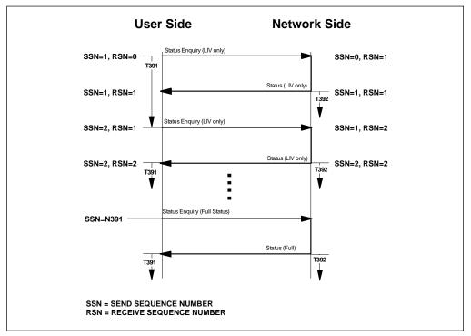
Figure 28. Link Integrity Verification Procedure. Status Enquiry(full) is used for link integrity verification as well.
