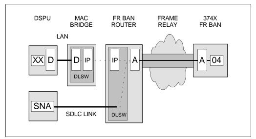
In both DLSw methods described previously, SNA data is transported in IEEE 802.2 LLC frames across the frame relay network.
