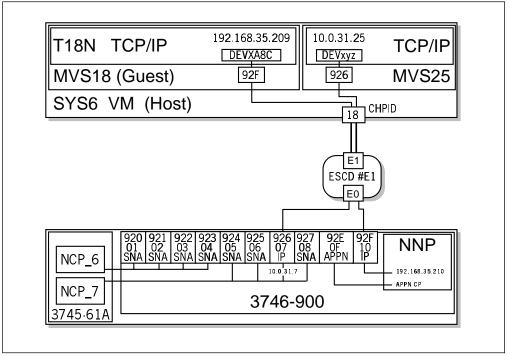
Figure 105. TCP/IP MVS ESCON Connection to the 3746-900 IP Router
