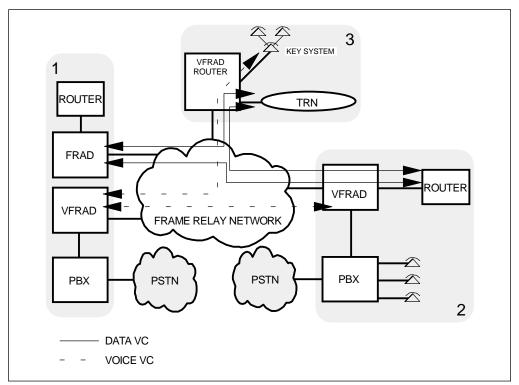
Figure 38. Voice over Frame Relay - Single and Dual Access
