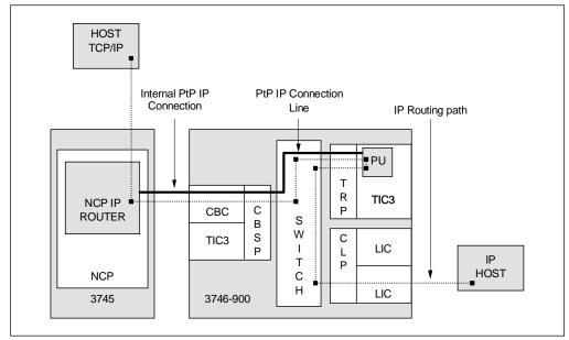
Figure 1. Internal IP PtP Connection
