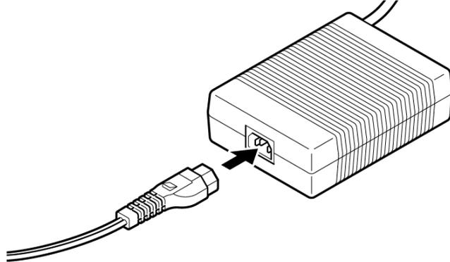
2. Connect the power plug to a properly grounded power outlet.
