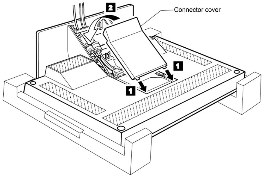
4. Reinstall the stand rear cover and turn the monitor to the upright position.
