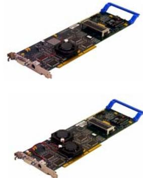
24-bit Z-buffer, 4/8-bit overlay, 8-bit double buffered Alpha, 8-bit stencil, up to 110MB texture memory, dual texture, and 3D texture. The GXT6500P has an additional geometry and lighting processor that further increases performance.
